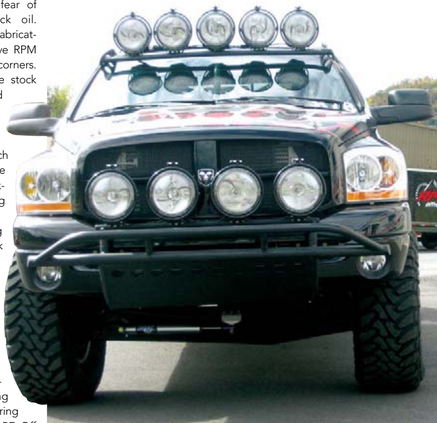
Each of the RPM Offroad race trucks is equipped with nine Baja Design Soltek 8-inch HID lights to cut through the Baja darkness.
