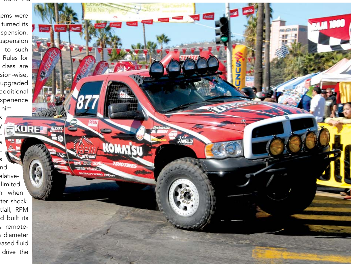
Each of the RPM Offroad race trucks is equipped with nine Baja Design Soltek 8-inch HID lights to cut through the Baja darkness.
